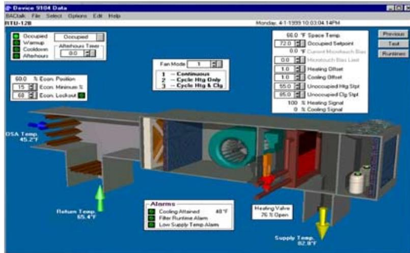
Alerton® Envision for BACtalk is powerful operator workstation software for BACnet systems. Use it to manage and control building equipment with unprecedented flexibility and power. Envision for BACtalk communicates with BACnet-compliant devices over an Ethernet LAN or through point-to-point (PTP) serial or modem connections.
